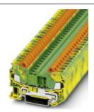
Ground modular terminal block, Connection method: Quick connection, Cross section: 0.5 mm² - 2.5 mm², AWG: 20 - 14, Width: 6.2 mm, Color: green-yellow, Mounting type: NS 35/7,5, NS 35/15
