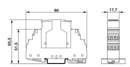
The figure shows the complete module consisting of a base element and connector
