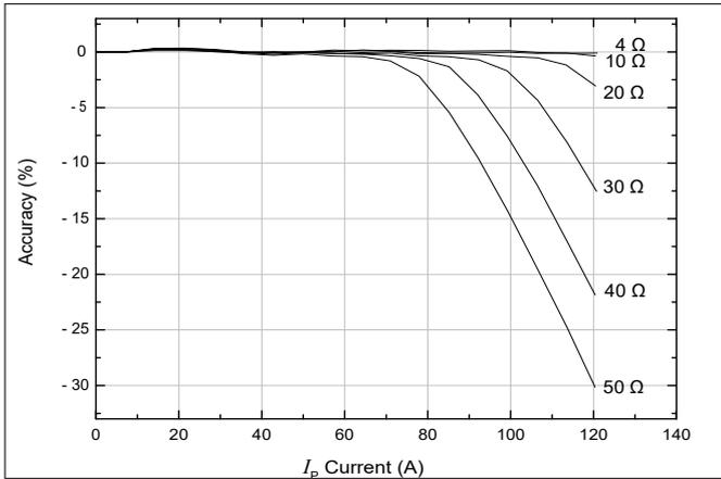
Figure 5: Accuracy vs.  $I_p$  Current @ 50 Hz
