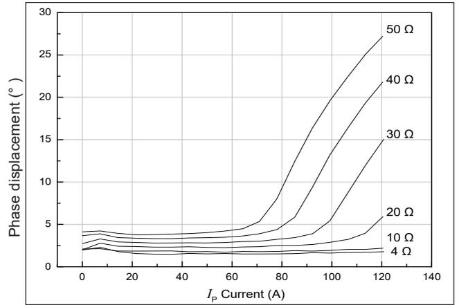
Figure 6: Phase displacement vs.  $I_p$  Current @ 50 Hz
