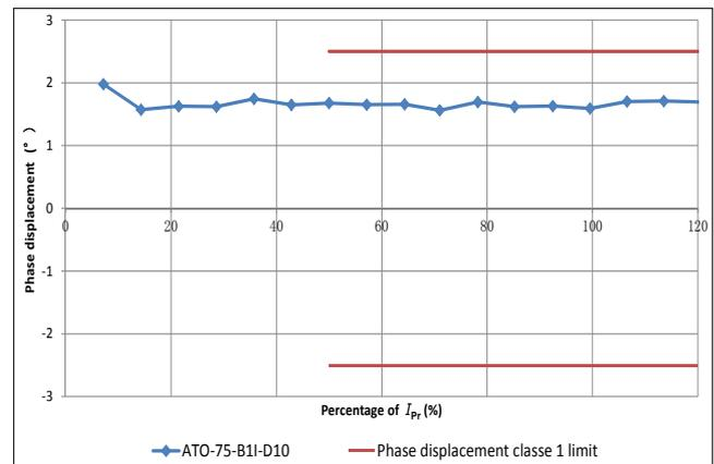
Figure 4: Phase displacement vs. Percentage of  $I_{Pr}$
