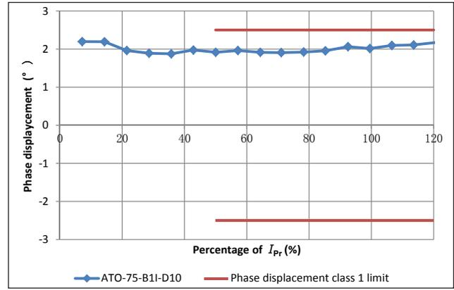
Figure 2: Phase displacement vs. Percentage of  $I_{Pr}$
