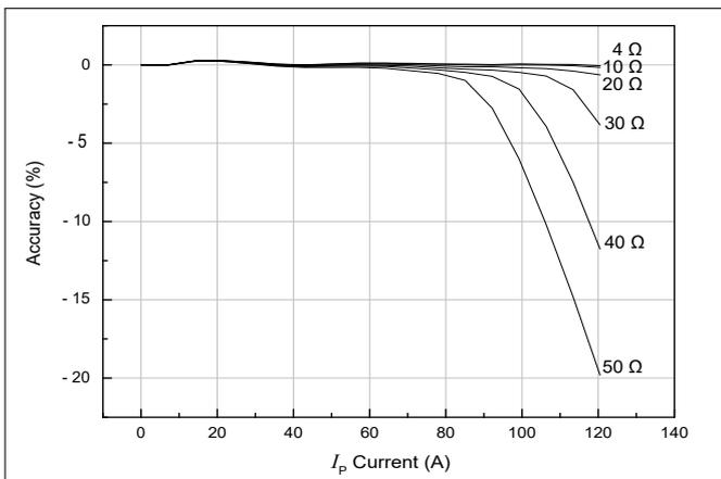
Figure 7: Accuracy vs.  $I_p$  Current @ 60 Hz
