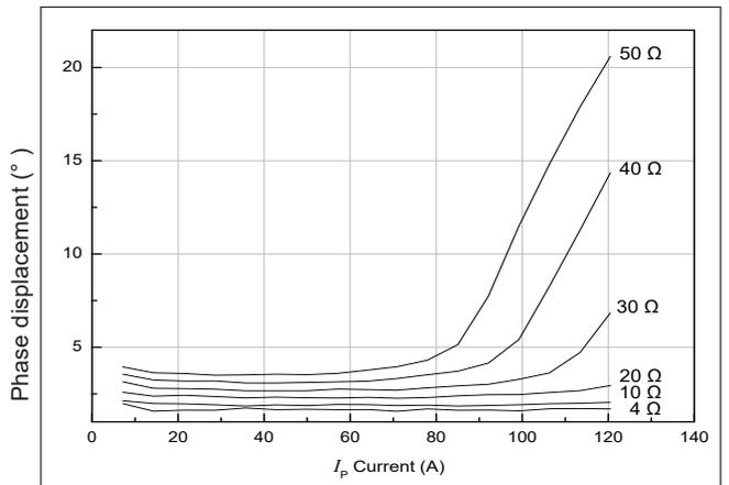
Figure 8: Phase displacement vs.  $I_p$  Current @ 60 Hz
