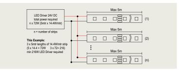
We recommend a maximum of 15mtrs strip per driver due to possible voltage drop
