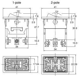
2. Dimensions of actuator: 1-pole: 12.6  $\times$  29, 2-pole: 17.4  $\times$  29
