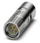
Cable connector, straight long, shielded: yes, Screw locking, M23, No. of pos.: 4+3+PE, type of contact: Pin, Crimp, cable diameter range: 7.5 mm ... 17 mm
