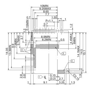
Note 1 Q indicates the center line of the microSD card slot.
