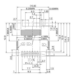
Q indicates the center line of the microSD card slot.
