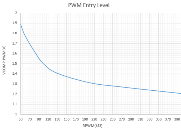
Figure 75. PWM Mode Entry Level Setting
