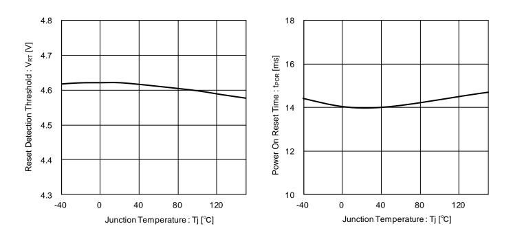
Figure 17. Reset Detection Threshold vs Temperature (RO: 10 k $\Omega$  pull-up to VO)
