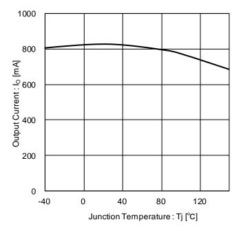
Figure 12. Output Current vs Temperature
