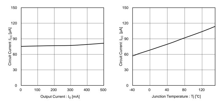
Figure 9. Circuit Current vs Output Current
