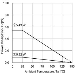
IC mounted on ROHM standard board based on JEDEC. ①: 1-layer PCB (Copper foil area on the reverse side of PCB: 0 mm × 0 mm) Board material: FR4 Board size: 114.3mm × 76.2mm × 1.57 mmt Mount condition: PCB and exposed pad are soldered. Top copper foil: ROHM recommended footprint + wiring to measure, 2 oz. copper. ②: 4-layer PCB (Copper foil area on the reverse side of PCB: 74.2 mm × 74.2 mm) Board material: FR4 Board size: 114.3mm × 76.2mm × 1.60 mmt
