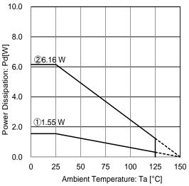
IC mounted on ROHM standard board based on JEDEC. ①: 1-layer PCB (Copper foil area on the reverse side of PCB: 0 mm × 0 mm) Board material: FR4 Board size: 114.3mm × 76.2mm × 1.57 mmt Mount condition: PCB and exposed pad are soldered. Top copper foil: ROHM recommended footprint + wiring to measure, 2 oz. copper. ②: 4-layer PCB
