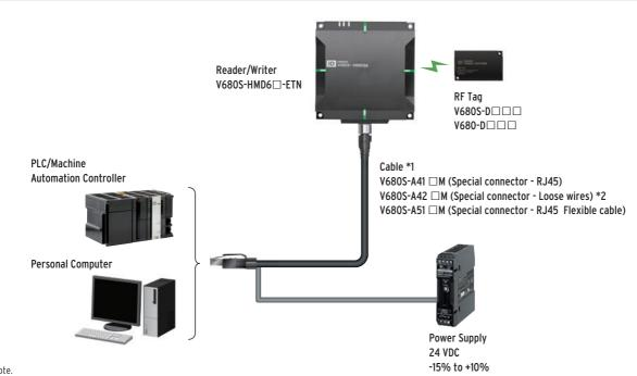
The cable can be extended up to 60 m by using the Extension Cable V680S-A40  $\square$ M (cable length: 10/20/50 m) or V680S-A50  $\square$ M (Flexible cable, cable length: 2/10/20m).
