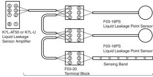
Total of 60 m max. (Sensing Band: 10 m max.) for the K7L-AT50 Total of 400 m max. for the K7L-U
