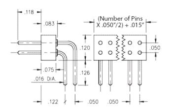
**Description:** Interconnect Header Right Angle Pin Header .016" (0,41mm) Pin Head Double Row Through Hole Plating Code: 10 Shell Plating: 10  $\mu$ " Gold over 100  $\mu$ " Nickel
