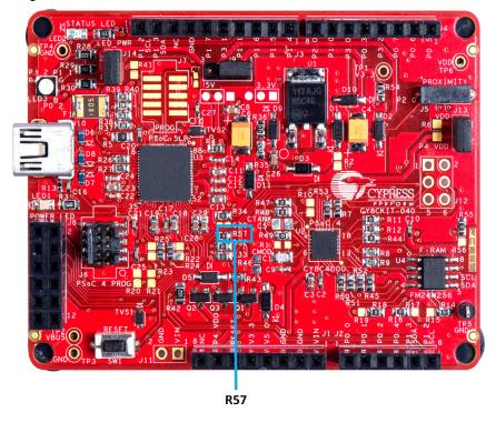
Figure 5-8. Debug Port Pin Functionality Selection
