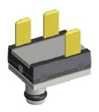
NovaSensor's NPR-101 pressure sensor is a silicon-based MEMS device using "Backside Absolute Pressure" technology designed for harsh media exposure, which eliminates the direct contact of the sensing circuitry with the applied media. The device is coupled with an ASIC to provide a ratiometric output proportional to the applied pressure. Integrated diagnostics included.
