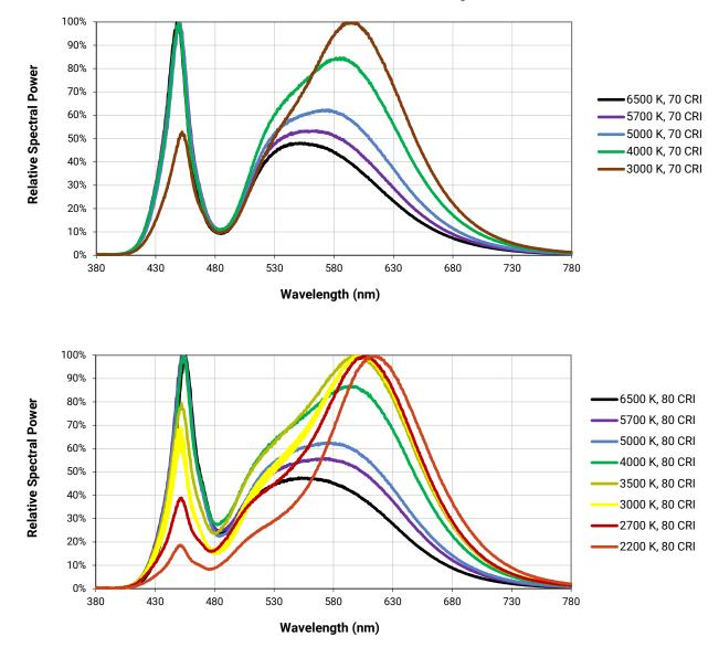
The following graphs are the result of a series of pulsed measurements at 1200 mA and T<sub>1</sub> = 85 °C.
