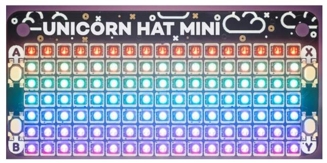
Over one hundred RGB LEDs, all individually-controllable, and four tactile buttons. It's the ultimate pocket-sized rainbow generator for Raspberry Pi!
