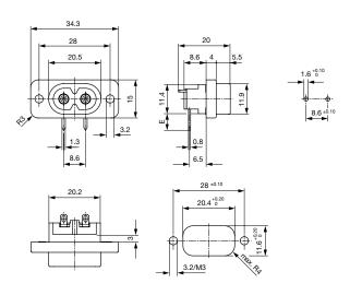
E = PCB terminal standard (additional solder): 6.9 mm
