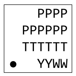
Figure 7.3. QFN40 Package Marking
