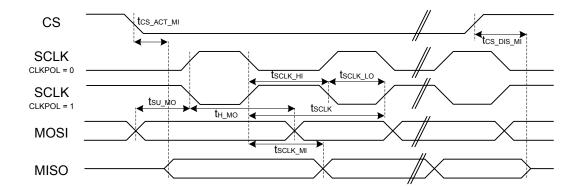
Figure 4.3. SPI Secondary Timing (SSSEARLY = 0)
