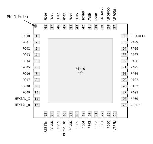
Figure 6.1. QFN48 / Standard Device Pinout
