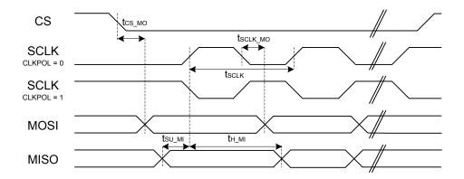
Figure 4.1. SPI Main Timing (SMSDELAY = 0)
