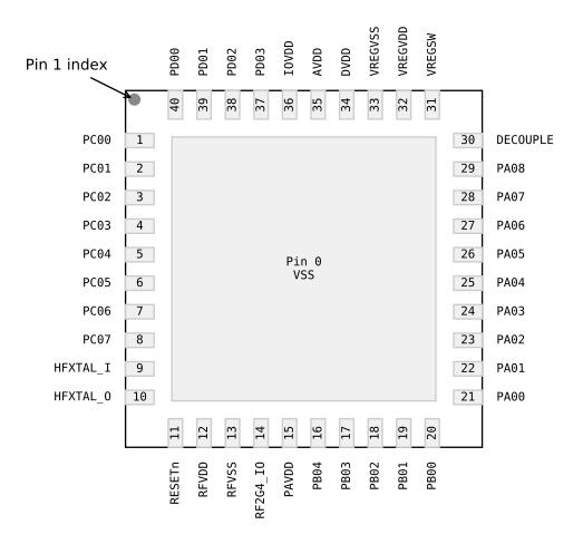
Figure 6.3. QFN40 / Standard Device Pinout
