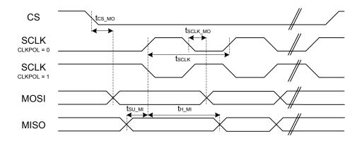
Figure 4.5. SPI Main Timing
