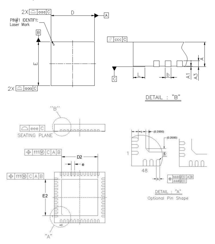
Figure 8.1. QFN48 Package Drawing
