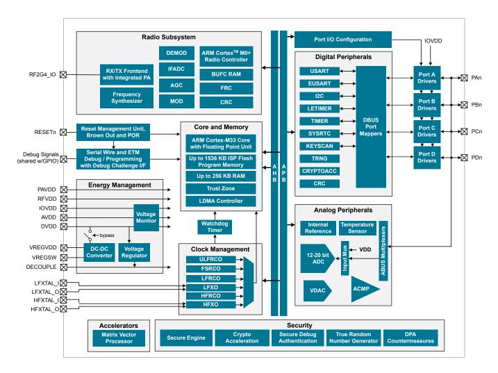
Figure 3.1. Detailed EFR32BG24 Block Diagram
