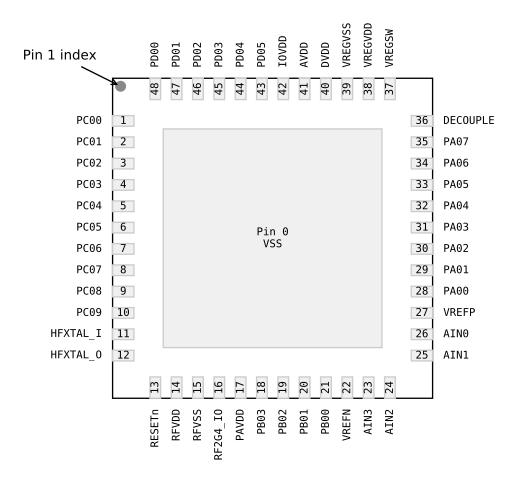
Figure 6.2. QFN48 / ADC Device Pinout
