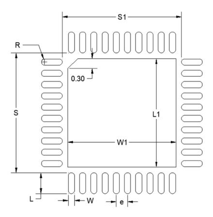
Figure 7.2. QFN40 PCB Land Pattern Drawing
