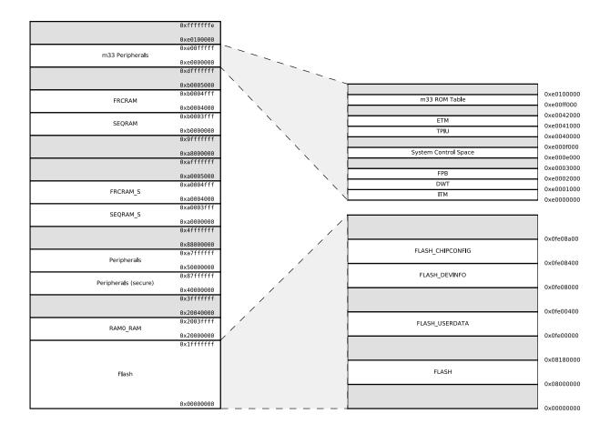
Figure 3.2. EFR32BG24 Memory Map — Core Peripherals and Code Space
