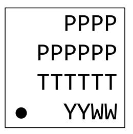
Figure 8.3. QFN48 Package Marking
