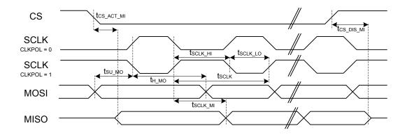
Figure 4.6. SPI Secondary Timing
