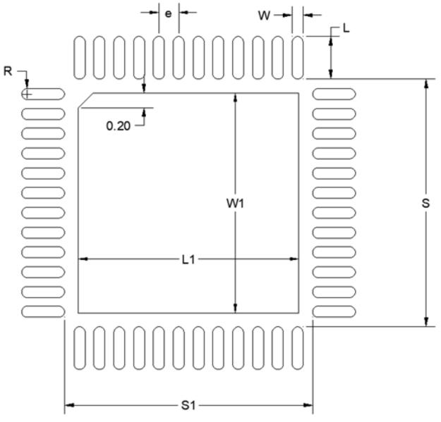
Figure 8.2. QFN48 PCB Land Pattern Drawing
