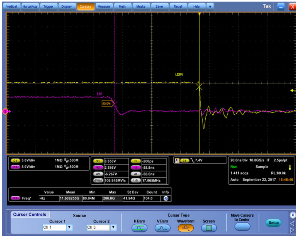
Figure 31. Low Side Turn-Off Propagation Delay (NCP51530A)
