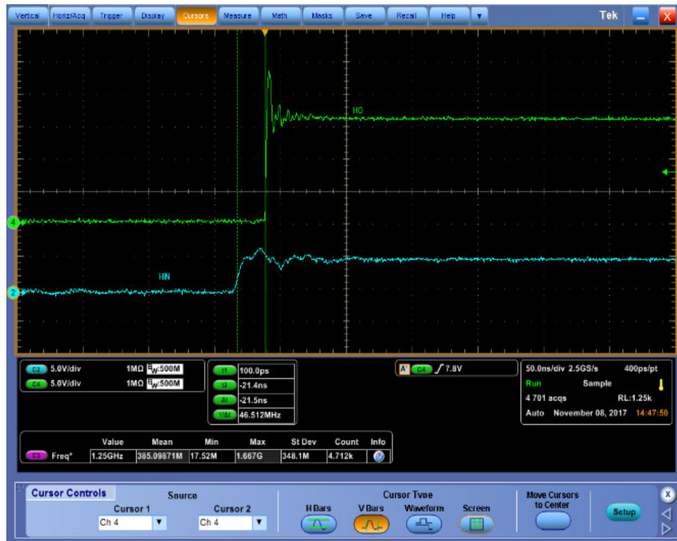
Figure 32. High Side Turn-Off Propagation Delay (NCP51530B)
