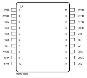
Figure 6-1. PW Package 20-Pin TSSOP Top View
