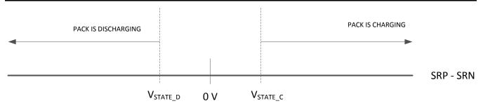
Figure 8-5. State Comparator Thresholds
