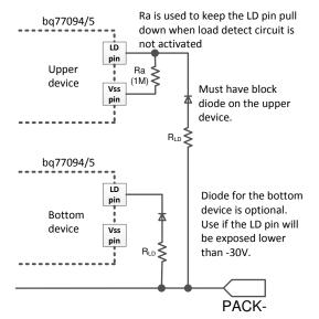
Figure 9-7. Simplified Circuit: LD Connection on Upper Device When Using for UV Fault Recovery
