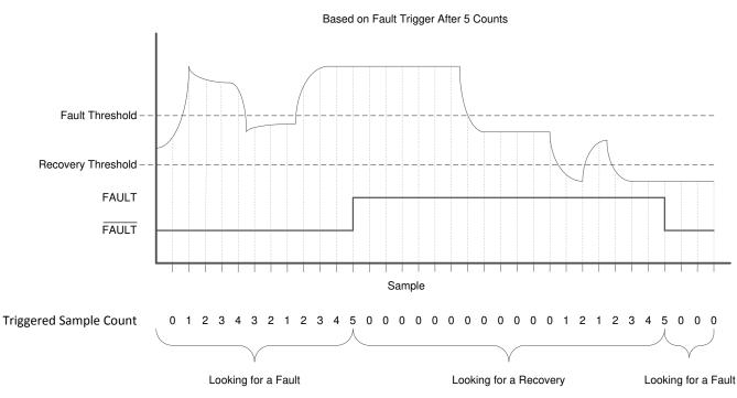
Figure 8-4. Fault Trigger Filtering
