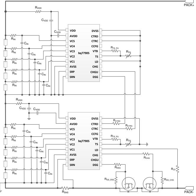
Figure 8-9. 10S Pack Using Two BQ77905 Devices
