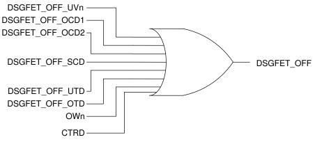
Figure 8-6. Faults that Can Qualify DSGFET\_OFF
