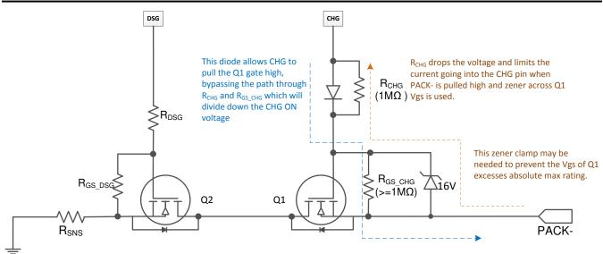
Figure 9-4. Protect CHG FET from a High Voltage on PACK-
