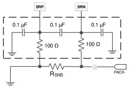
Figure 9-8. Optional Filters Improve Current Measurement
