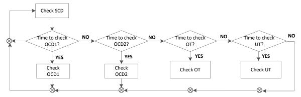
Figure 8-2. Comparator 2 Flowchart
