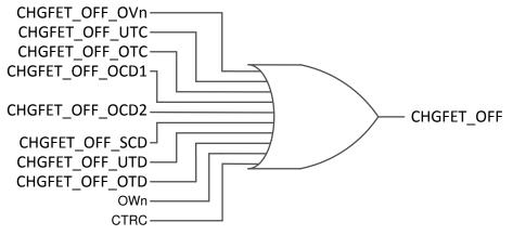
Figure 8-7. Faults That Can Qualify CHGFET OFF
