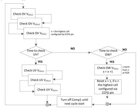
Figure 8-1. Comparator 1 Flowchart
