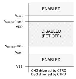
Figure 8-8. External Override of CHG and DSG Drivers
