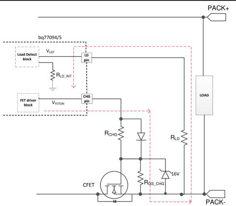
Figure 9-6. Load Detect Circuit During UV Fault
