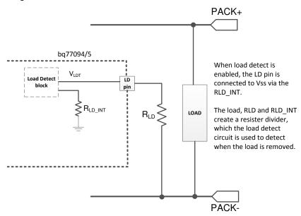
Figure 8-3. Load Detection Circuit for Current Faults Recovery
