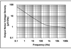
**FIGURE 2-13:** Output Noise Voltage Density ( $V_{REF}$  Noise Density) vs. Frequency. Gain = 1x.
