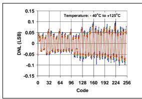
FIGURE 2-9: DNL vs. Code and Temperature (MCP4801).
