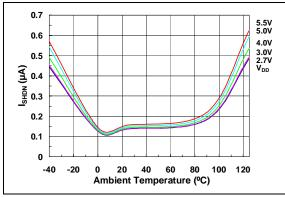
**FIGURE 2-18:** Hardware Shutdown Current vs. Temperature and V<sub>DD</sub>.
