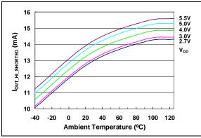
**FIGURE 2-27:**  $I_{OUT}$  High Short vs. Temperature and  $V_{DD}$ .
