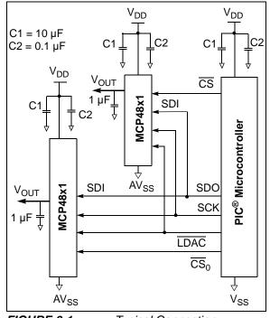
FIGURE 6-1: Typical Connection Diagram.
