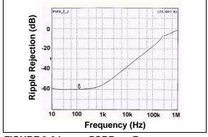
FIGURE 2-34: PSRR vs. Frequency.
