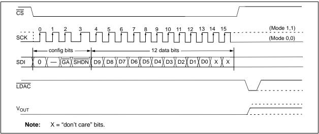
FIGURE 5-2: Write Command for MCP4811 (10-bit DAC).
