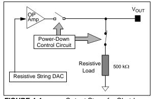
FIGURE 4-4: Output Stage for Shutdown Mode.
