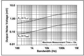
**FIGURE 2-14:** Output Noise Voltage (V<sub>REF</sub> Noise Voltage) vs. Bandwidth. Gain = 2x.
