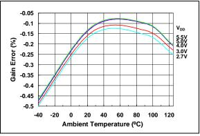
**FIGURE 2-21:** Gain Error vs. Temperature and V<sub>DD</sub>.
