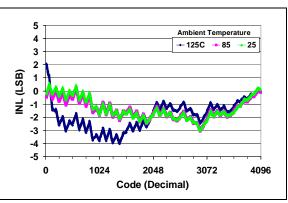
FIGURE 2-4: INL vs. Code and Temperature (MCP4821).
