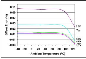
**FIGURE 2-20:** Offset Error vs. Temperature and V<sub>DD</sub>.
