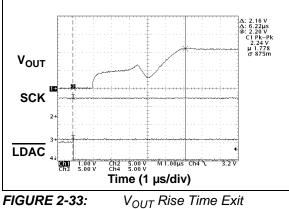
FIGURE 2-33: V<sub>OUT</sub> Rise Time Exi Shutdown.
