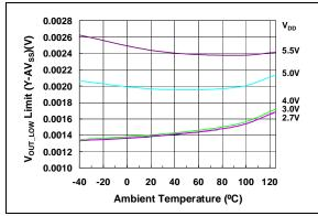
**FIGURE 2-26:** V<sub>OUT</sub> Low Limit vs. Temperature and V<sub>DD</sub>.
