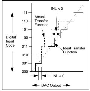
FIGURE 4-1: Example for INL Error.
