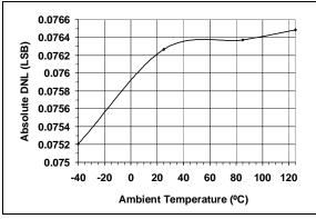
FIGURE 2-3: Absolute DNL vs. Temperature (MCP4821).
