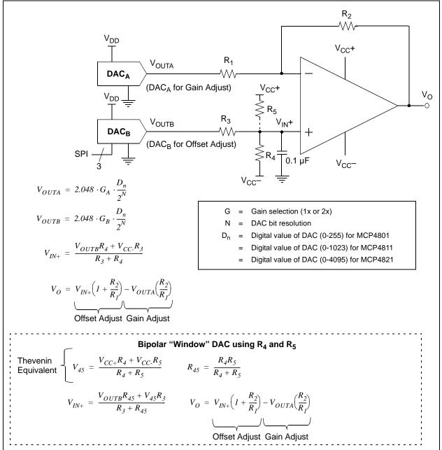
EXAMPLE 6-4: BIPOLAR VOLTAGE SOURCE WITH SELECTABLE GAIN AND OFFSET
