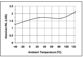
FIGURE 2-5: Absolute INL vs. Temperature (MCP4821).
