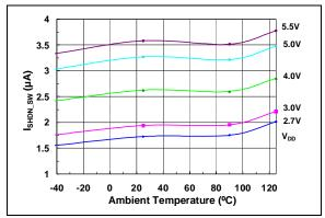
**FIGURE 2-19:** Software Shutdown Current vs. Temperature and V<sub>DD</sub>.
