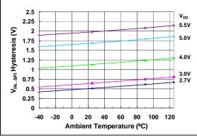
**FIGURE 2-24:** Input Hysteresis vs. Temperature and V<sub>DD</sub>.
