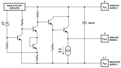
Figure 11. Simplified schematic diagram.
