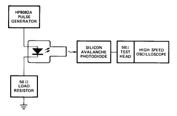
Figure 12. Test circuit for measuring  $\,t_{r_{\rm f}}\,t_{\rm f}$ .
