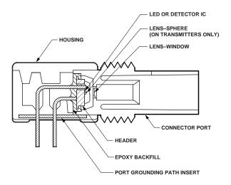
Figure 1. HFBR-0400 ST series cross-sectional view.
