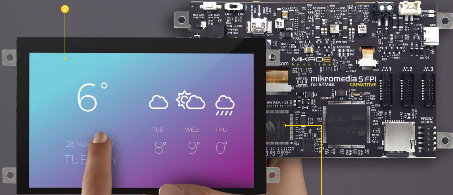
Figure 10: Display and SSD1963 view
