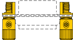
K Rotating male jackscrews, low-profile, internal hex, 36-position polarization (mates to S jackpost)
