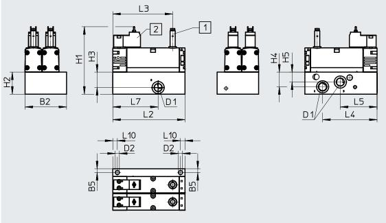
[1] Proximity switch PNP or NPN, size M8x1, plug connection to EN 61076-2-104 [2] Electrical connection to EN 175301-803, type C
