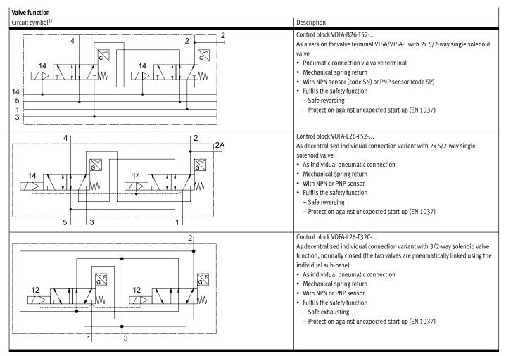
1) The symbol represents a valve with a proximity switch with a switching output signal, in the illustration an N/O contact. In accordance with ISO 1219-1, this symbol applies to both N/O contacts and N/C contacts. The switching element function of all sensors used here is an N/C contact.
