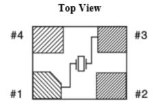
Pin #1: Crystal Pin #3: Crystal Pin #2: GND (\*)
