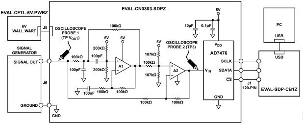
Figure 8. Test Setup Functional Block Diagram
