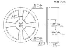
Note: Dimensions of items produced after December 2006 bilinerisbins of items produced after beceininer 2006 have changed as shown below.  $100^{24}$  dia.  $3.93^{2.039}$  dia.  $\rightarrow 80^{24}$  dia.  $3.150^{1.039}$  dia.;  $370^{22}$  dia.  $14.567^{1.079}$  dia.  $\rightarrow 380^{22}$  dia.  $14.961^{1.079}$  dia.
