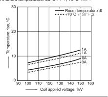
5-(2). Coil temperature rise Tested sample: TXS2-24V, 6 pcs.
