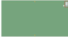
PCB size: 120mm x 65mm x 1mm Antenna area: 8 x 5 mm
