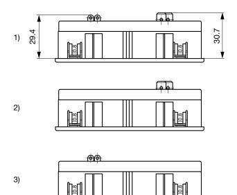
1) Solder and quick connect terminals 6.3x0.8 mm
