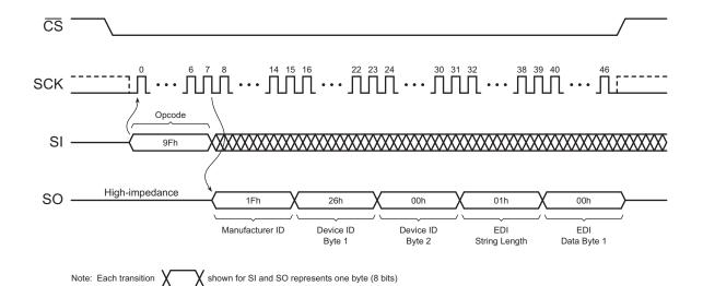
Figure 48. Manufacturer and Device Read (Opcode 9Fh)
