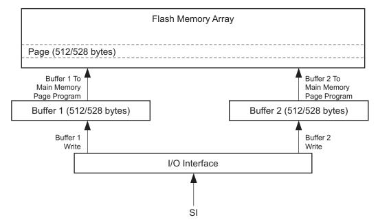
Figure 31. Block Diagram
