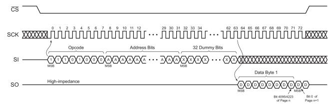
Figure 38. Continuous Array Read (Legacy Opcode E8h)
