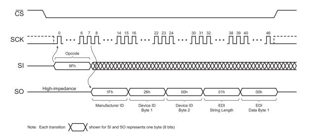
Figure 21. Read Manufacturer and Device ID
