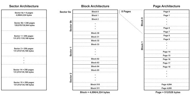
Figure 3. Memory Architecture Diagram
