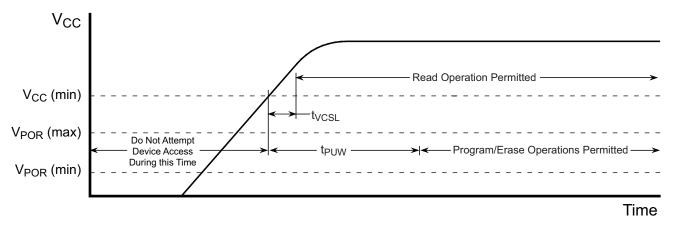
Figure 23. Power-Up Timing
