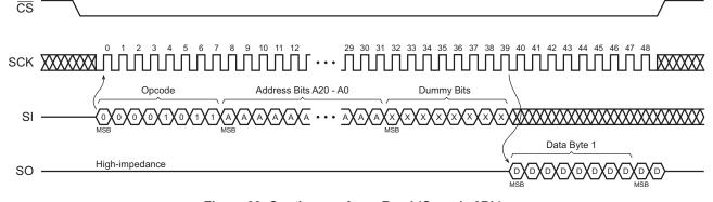
Figure 39. Continuous Array Read (Opcode 0Bh)
