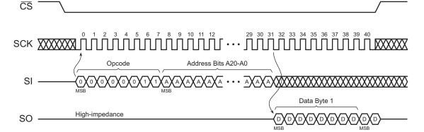
Figure 40. Continuous Array Read (Opcode 01h or 03h)
