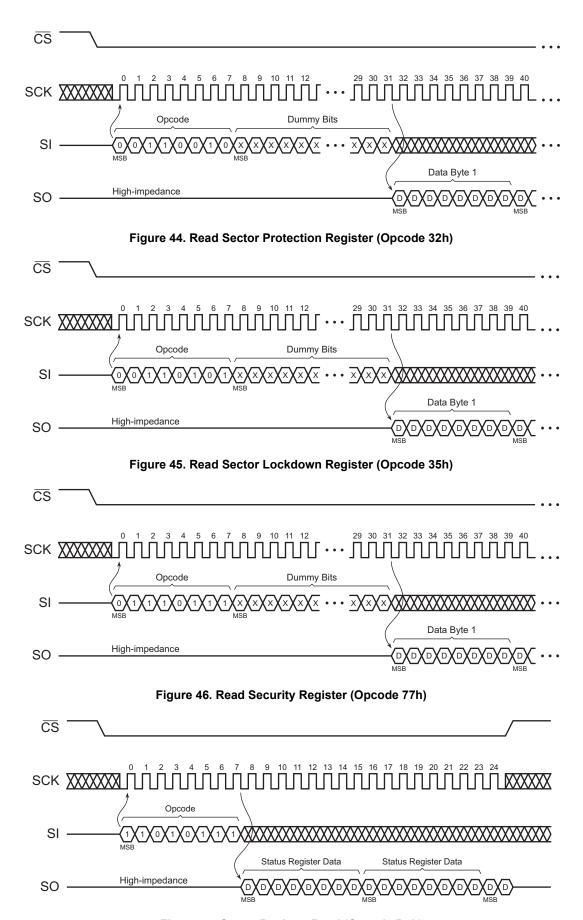
Figure 47. Status Register Read (Opcode D7h)
