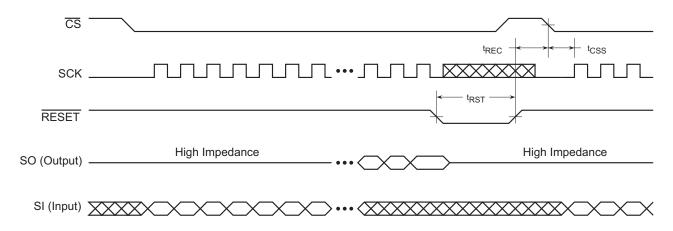
Figure 49. Reset Timing
