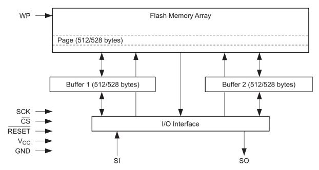
Figure 2. Block Diagram
