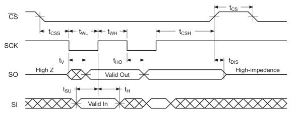
Figure 28. Waveform 2 = SPI Mode 3 Compatible
