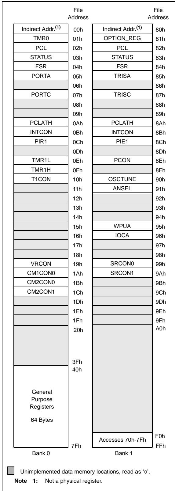
FIGURE 2-3: DATA MEMORY MAP OF THE PIC16F610/16HV610
