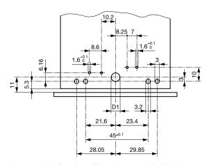
Fixation on PCB or housing from below
