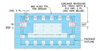
NOTE: 1. COPLANAR WAVEGUIDE PARAMETERS ARE SHOWN FOR ROGERS RO4350B WITH DIELECTRIC THICKNESS .060" ± .004";
