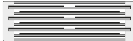
Extended metallized film design with internal series connection (series connection of 2 elements)
