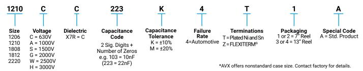
Notes: Capacitors with X7R dielectrics are not indeded for applications across AC supply mains or AC line filtering with polarity reversal. Please contact AVX for recommendations
