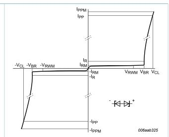
V-I characteristics for a bidirectional ESD Fig. 4. protection diode
