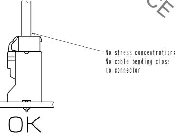
2) When applying load to connector end, please use the retainer for reducing the stress affection on the connector. Retainer shall be installed after inserted crimping contact completely. It might be impossible to insert it when terminal installation is incompleted.
