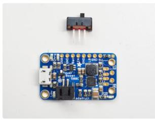
The switch will go into the breakout header, and attach to VBAT EN and GND The switch is symmetric so as long as those three pins are attached to the switch you are good to go
