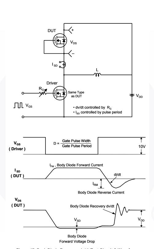
Figure 17. Peak Diode Recovery dv/dt Test Circuit & Waveforms
