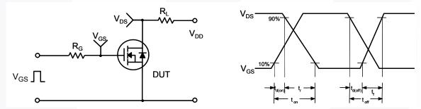
Figure 15. Resistive Switching Test Circuit & Waveforms
