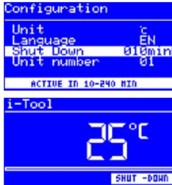
The adjustable shut-down function (idle state) serves the purpose of energy saving and prolonging the lifetime of soldering tip and heater. In idle state the tools cool down to room temperature. The bottom line in the display then shows the text [Shut Down]. You can end the idle state at any time by actuating the i-OP.
