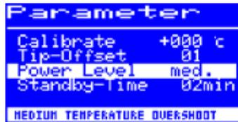
This function enables the user to influence the regulating behavior of the station, whereby the heating and after heating behavior of the station can be matched to the actual application. Three settings are possible: [high], [med.] and [low].
