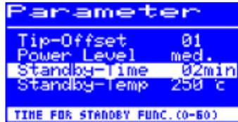
The standby period is the time from the last work with the soldering tool to the point when the standby temperature is activated. The setting range is between 20 seconds and 60 minutes. The input [0] deactivates the standby function.
