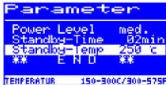
This is the soldering tip temperature during work breaks. It is automatically activated when the standby-time has elapsed. When the temperature is decreased, power is saved and the service life of tip and heating element is increased.
