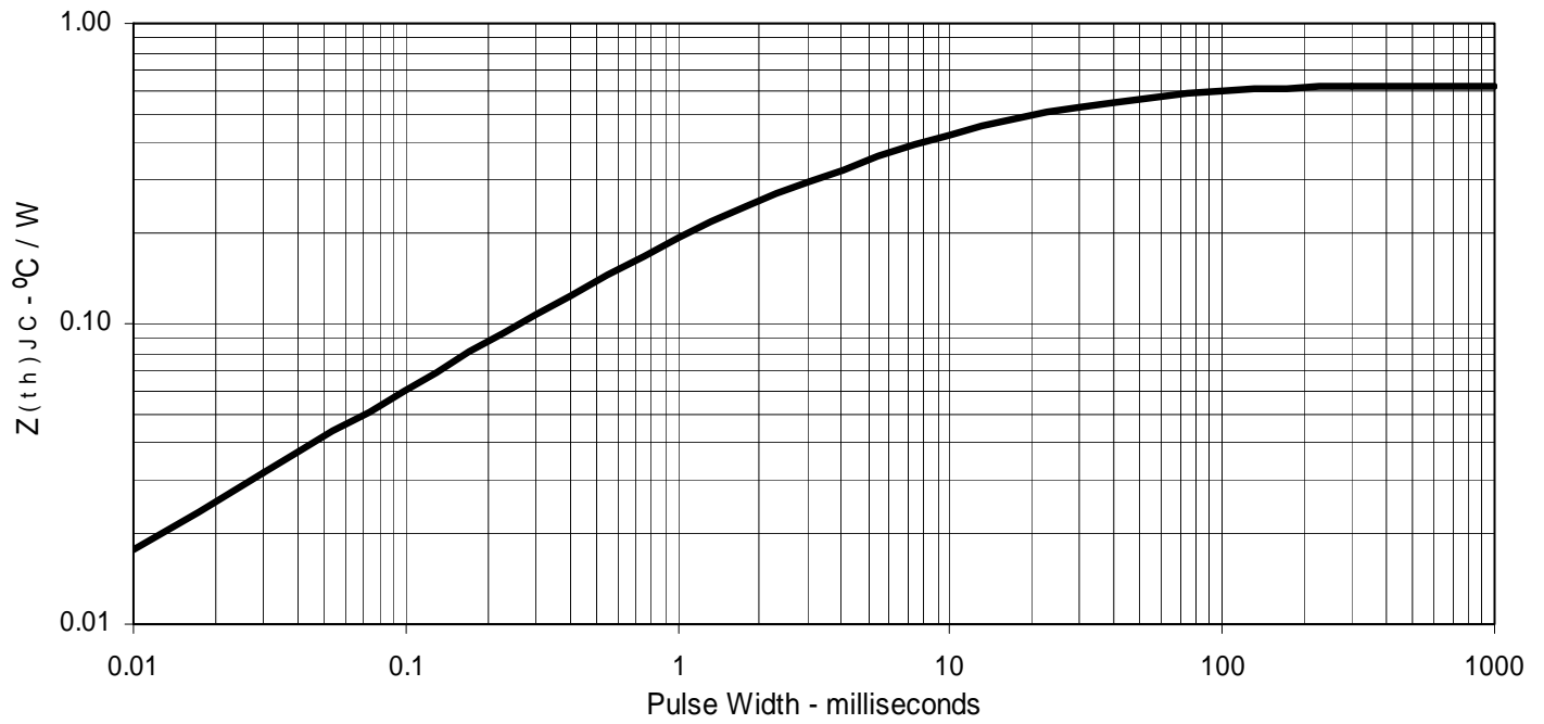
Fig. 13. Maximum Transient Thermal Impedance
