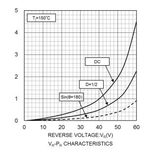
REVERSE POWER DISSIPATION:P<sub>R</sub>(W)
