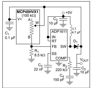
FIGURE 8-7: Programmable Power Supply.
