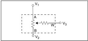
FIGURE B-1: POTENTIOMETER CONFIGURATION.
