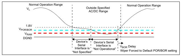
FIGURE 4-4: Power-Up and Brown Out - V+/V- at Normal Operating Voltage.
