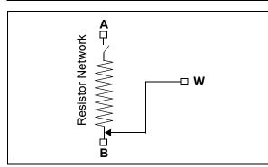
FIGURE 4-5: Hardware Shutdown Resistor Network Configuration.
