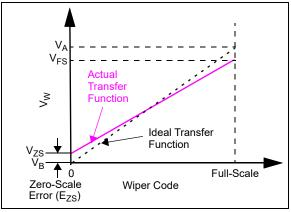
FIGURE B-6: ZERO-SCALE ERROR EXAMPLE.
