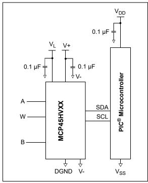
FIGURE 8-13: Typical Microcontroller Connections.
