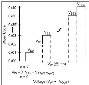
FIGURE B-3: THEORETICAL V<sub>W</sub> OUTPUT VS CODE (MONOTONIC OPERATION).
