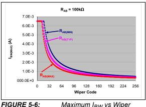
**FIGURE 5-6:** Maximum  $I_{BW}$  vs Wiper Code - 100 k $\Omega$ .
