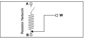
**FIGURE 5-11:** Resistor Network Shutdown State (R0HW = 0).
