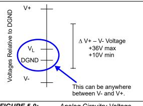
*FIGURE 5-9:* Analog Circuitry Voltage Ranges.
