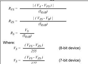
$\mathbf{V_{FS}}$  is the V<sub>W</sub> voltage when the wiper code is at full scale.
