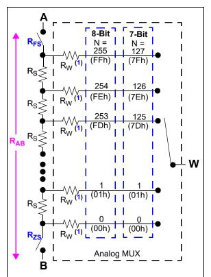
Note 1: The wiper resistance is dependent on several factors including wiper code, device V+ voltage, terminal voltages (on A, B and W), and temperature. Also for the same conditions, each tap selection resistance has a small variation. This  $R_W$  variation has greater effect on some specifications (such as INL) for the smaller resistance devices (5.0 k $\Omega$ ) compared to larger resistance devices (100.0 k $\Omega$ ).
