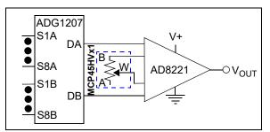
*FIGURE 8-4:* Variable Gain Instrumentation Amplifier for Data Acquisition System.
