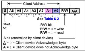
**FIGURE 6-9:** Client Address Bits in the l<sup>2</sup>C Control Byte.
