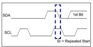
FIGURE 6-5: Repeat Start Condition Waveform.
