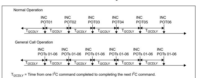
**FIGURE 8-12:** Example Comparison of "Normal Operation" vs. "General Call Operation" Wiper Updates.
