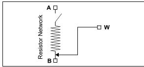
FIGURE 5-10: Hardware Shutdown Resistor Network Configuration.
