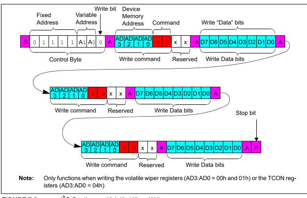
FIGURE 7-3: I<sup>2</sup>C Continuous Volatile Wiper Write.
