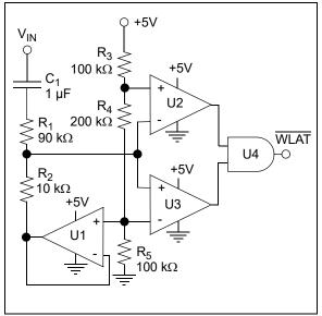
FIGURE 8-6: Referenced Voltage Crossing Detect.
