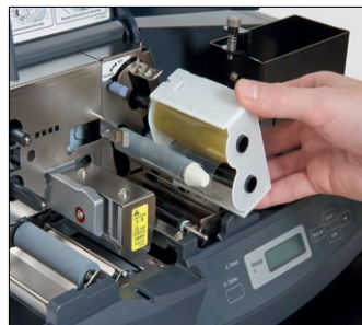
Special cleaning cassette easy to remove
