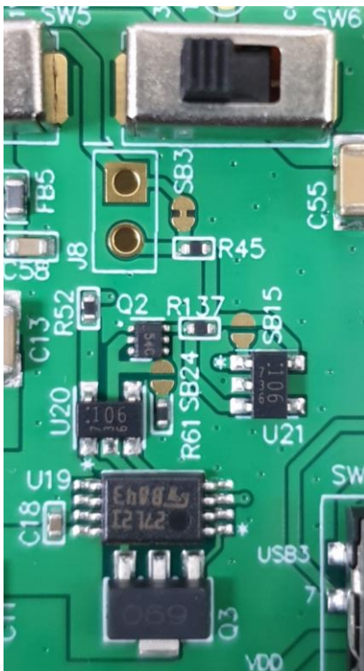
Figure 5: Schematic and PCB location of SB24
