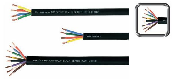
Van Damme Black Series Tour Grade Speaker Cable offers a comprehensive conductor size and core count to accommodate almost all potential speaker signals. From 2 core 1.5mm through 8 core 4mm to 18 core 2.5mm the ultra pure copper conductors, cutting edge PVC compounds and dynamic use focused construction provide accurate signal transmission, toughness and flexibility.
