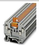
Knife disconnect terminal block with two-sided double connection, cross section: 0.2 - 2.5 mm², AWG: 30 - 10, width: 6.2 mm, color: gray
