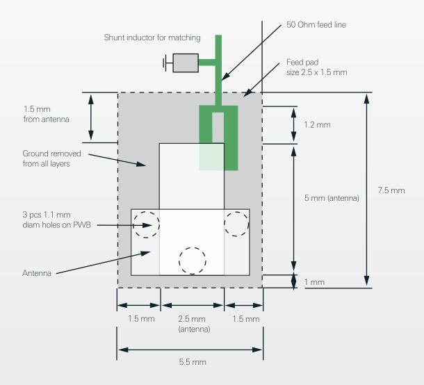
Matching and tuning component values depend on application and surrounding mechanics / materials.
