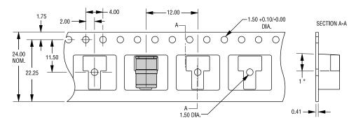
TOLERANCES: ±0.13 UNLESS OTHERWISE SPECIFIED DIMENSIONS: MILLIMETERS
